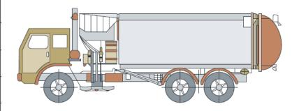
This is the most commonly used vehicle for domestic garbage and recycling collections. It is only suitable for collecting MGBs up to 360 litres in size.
